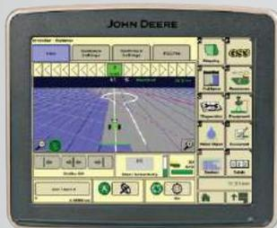
iTEC Pro is used with the StarFire 3000 Receiver and GreenStar 3 2360 Display.
