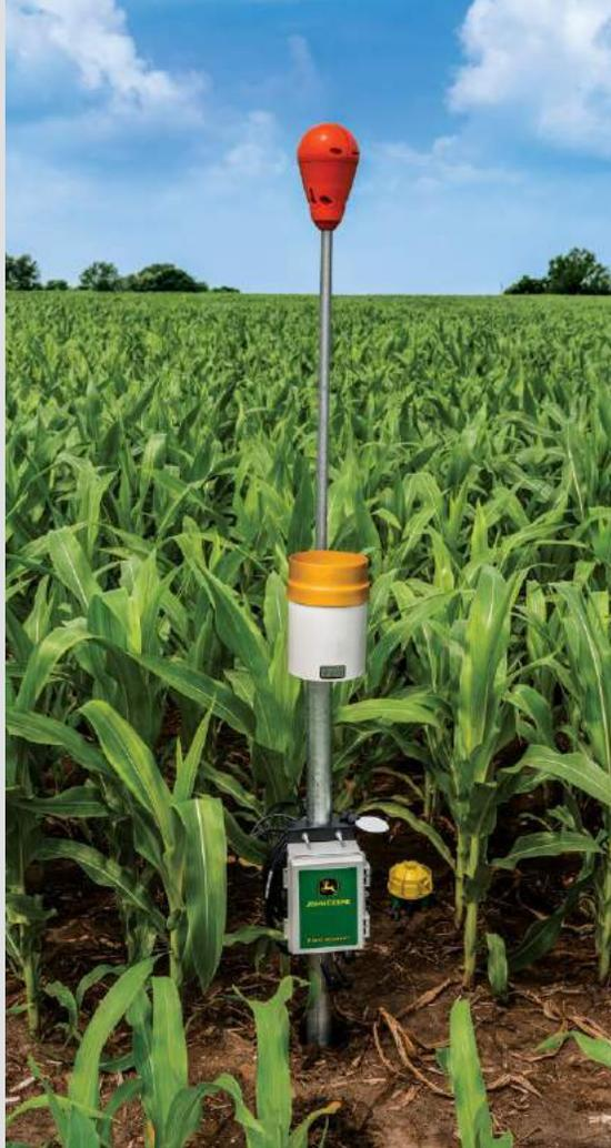
Wireless radio kits let you install up to eight different probes in different parts of your field, tied to a single gateway. Not only does this significantly reduce overall costs, it gives you a much clearer picture of your field, including different soil types that may require different irrigation strategies. With 3G coverage, you can install up to eight probes within a mile of a gateway; with satellite coverage, up to 3 probes within a mile.
