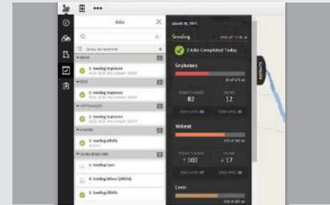
**Remote Display Access** lets you and your trusted partners remotely view an operator's screen, to resolve issues or make changes without making a trip to the field. Your dealer can also reduce downtime by reading diagnostic codes remotely, as well as recording performance readings. See pages 34-35.
