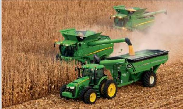
John Deere Machine Sync allows a combine operator to automatically control the location of a tractor and grain cart while unloading on-the-go, which is not only a time-saver, it lets you put more grain in the cart, with less spillage.
