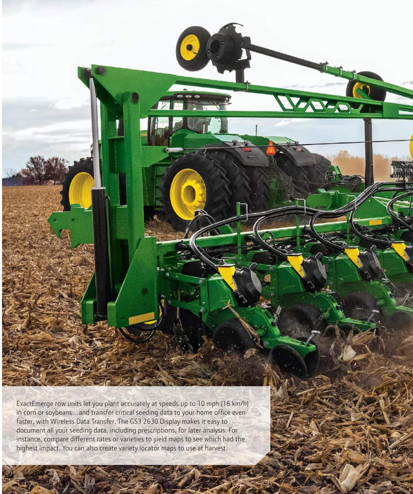
ExactEmerge row units let you plant accurately at speeds up to 10 mph (16 km/h) in corn or soybeans... and transfer critical seeding data to your home office even faster, with Wireless Data Transfer. The GS3 2630 Display makes it easy to document all your seeding data, including prescriptions, for later analysis. For instance, compare different rates or varieties to yield maps to see which had the highest impact. You can also create variety locator maps to use at harvest.
