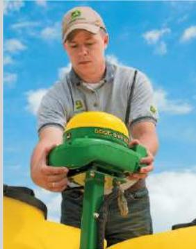
Guidance starts with a StarFire Receiver. You can choose the accuracy you need, ranging from plus-or-minus 9 inches (recommended for many broad acre applications) down to sub-inch accuracy with RTK.
