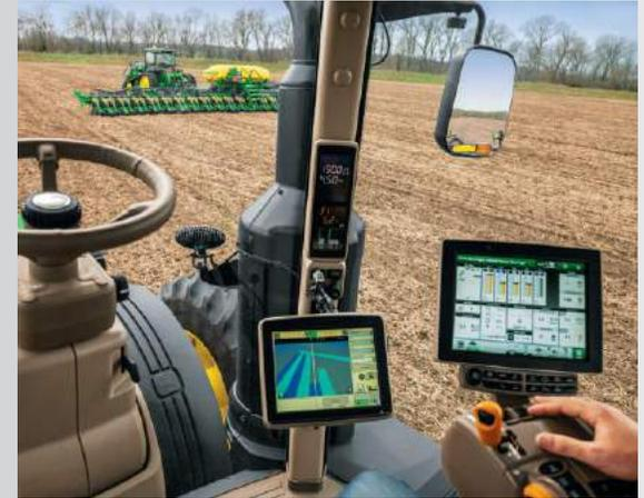
Machine Sync allows coverage map sharing and guidance line sharing to improve planting, seeding, spraying and nutrient application. This increases efficiency in the field, because two machines can work simultaneously with each operator having immediate access to coverage maps and guidance lines to ensure complete field coverage. Use Machine Sync in tandem with Section Control to ensure you're not overlapping at any point, which wastes seed (and money).
