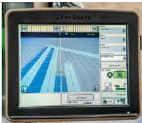
John Deere Machine Sync provides operators of combines and tractors logistical information never before available. From a single map view on the GreenStar™ 3 2630 Display, operators are able to view up to ten machines operating within a single network.
