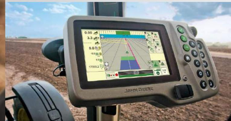
The GreenStar™ 2 1800 Display is a 7-inch full-color display with a simple interface and smaller price tag. You can easily toggle between multiple home pages to monitor more than one in-field activity and navigate through fields with greater control and confidence.
