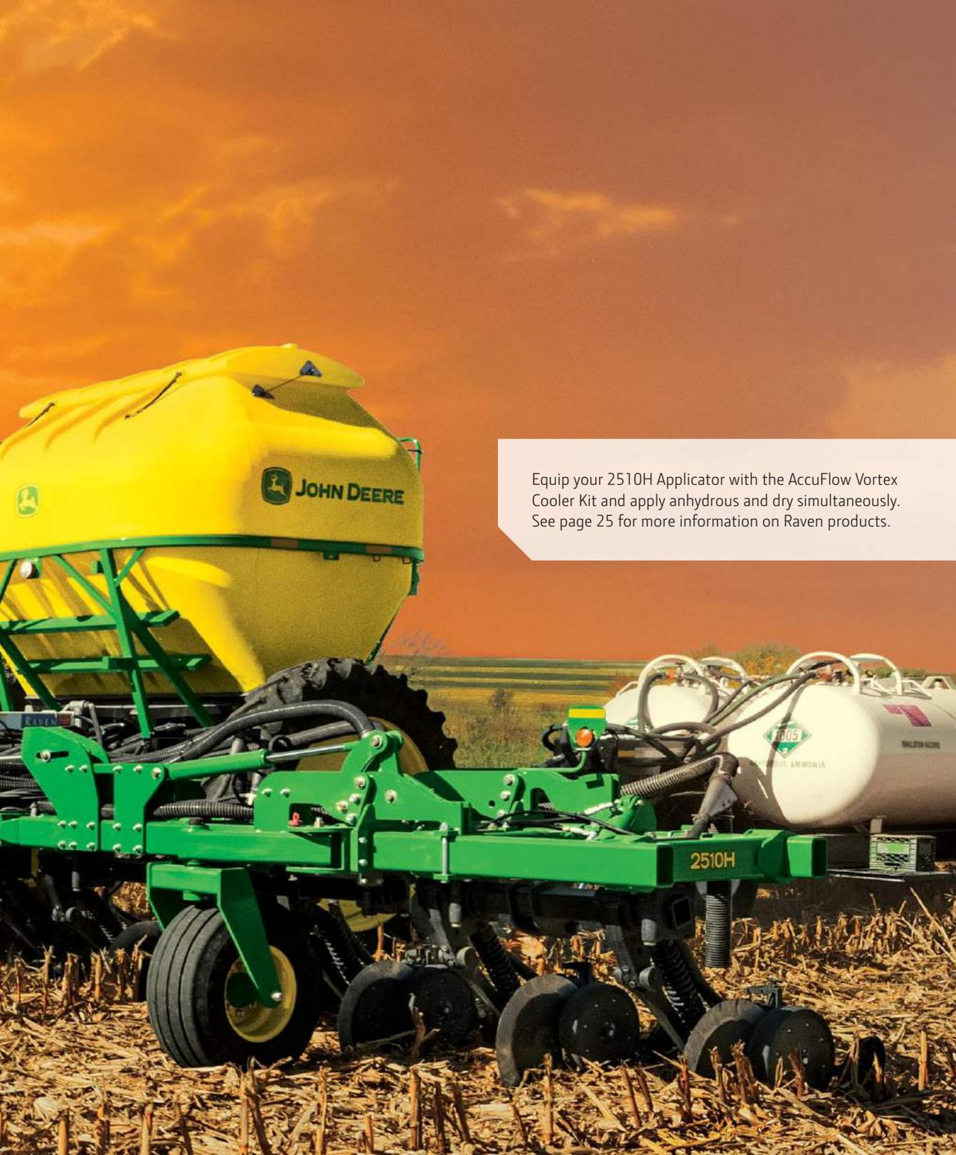
Equip your 2510H Applicator with the AccuFlow Vortex Cooler Kit and apply anhydrous and dry simultaneously. See page 25 for more information on Raven products.
