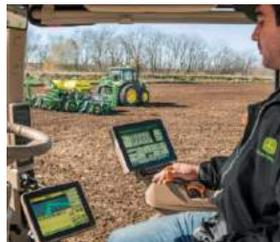
When you pair Section Control with Machine Sync, you can run multiple planters in the same field and save both time and seed. Section Control automatically turns sections off and on based on another machine's coverage, so you'll have peace-of-mind knowing that you didn't waste seed on headlands, or overlapping passes.
