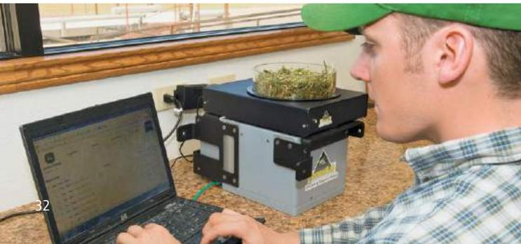
**The HarvestLab moisture sensor** uses Near-Infrared Technology (NIR) for accurate readings that aren't affected by humidity or atmospheric conditions. You'll get instantaneous moisture data, as well as yield data, that can be used in the cab to make informed decisions during harvest. The information can also be stored for later analysis and reporting.
